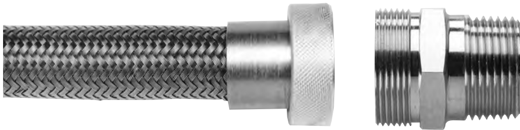
P/N 22037 (Plated) Adapter 1 3/16"-18 UNEF x 3/4"-14 NPT
