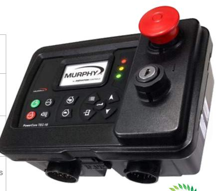
Murphy's PowerCore® TEC-10 panel provides full control of your engine including auto start/stop, auto throttling and display of engine parameters along with critical faults from the engine/application. The TEC-10 supports SAE J1939 CAN protocols for electronically governed engines as well as analog sensors on mechanical engines for fault and safety warnings/shutdowns.
